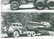
The armored M26 was based on a mining truck design; in military service, it could be armed (note Car and Foundry the MG ring on the r Works of Renton those, which described the tractor as the Model TR-1. and measured 25 ft. 4 in. long, 10 ft. 10 in. wide, and 11 ft. 5 in
