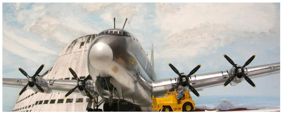
The Lockheed R6V was Moffett Field's big deal in 1949. In the nose wheel well, an aluminum ladder could be pulled down that allowed passengers and crew to enter and exit to the lower deck.
