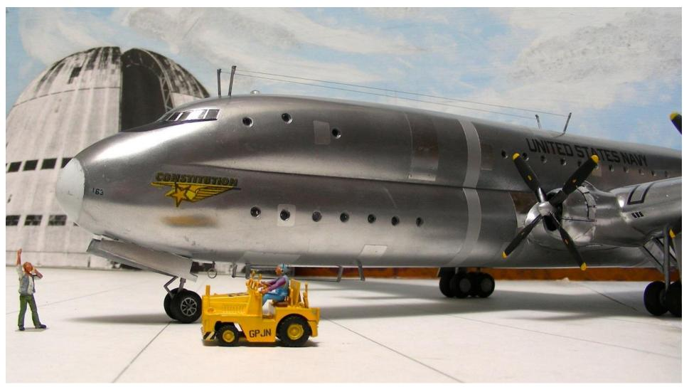
The world's most under-powered monster viewed up close and personal. The four Pratt & Whitney R-4360-22W 28 cylinder aircooled Wasp Major engines, producing 3250 HP weren't up to the task. To get this thing up in the air with a payload, it needed a boost. With full take-off power, six JATO bottles were fired just long enough to get the wheels retracted. With their drag eliminated, the R6V managed to climb above tall buildings.
