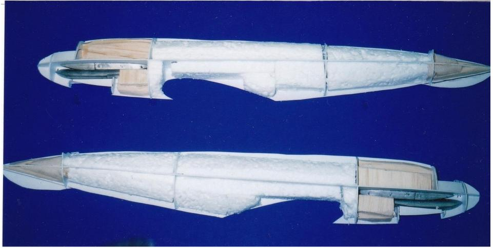
2- Fuselage patterns cut from .030 styrene sheet with thickness templates glued into place, and filled with styrofoam and balsa to reduce the amount of resin putty, thus saving weight and money. Lead weights are glued in the nose for balance.
