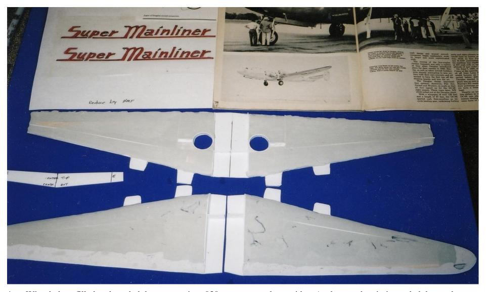
4- Wing halves filled and sanded down exposing .030 styrene template guides. As the cured resin is sanded down, the templates show through and you stop sanding. This is a high energy build.
