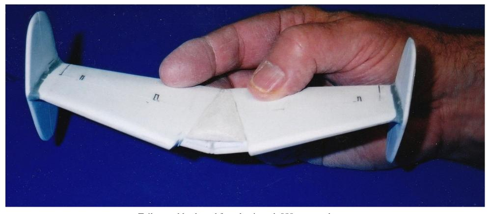
Tail assembly shaped from laminated .080 styrene sheet
