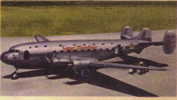
PERFORMANCE — Powered with four Pratt & Whitney twin-row "Hornet" engines developing 1100 h.p. each, the DC-4 has a maximum speed of 257 m.p.h., a cruising speed of 235 m.p.h. and a cruising range of 2600 miles. Rate of climb 1200 ft./min. Service ceiling 22,900 ft. Manufactured by Douglas Aircraft Corporation, Santa Monica, California.
