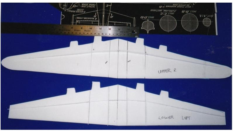
1- Patterns cut from .030 styrene sheet. Thickness templates glued in place. Lower wing pattern cut short chordwise to allow sharp trailing edges. Tips are cut short for the same reason. Also pictured is the copy of the Douglas factory drawing for a scale model of the DC-4 for sales purposes (via Mike Herrill)
