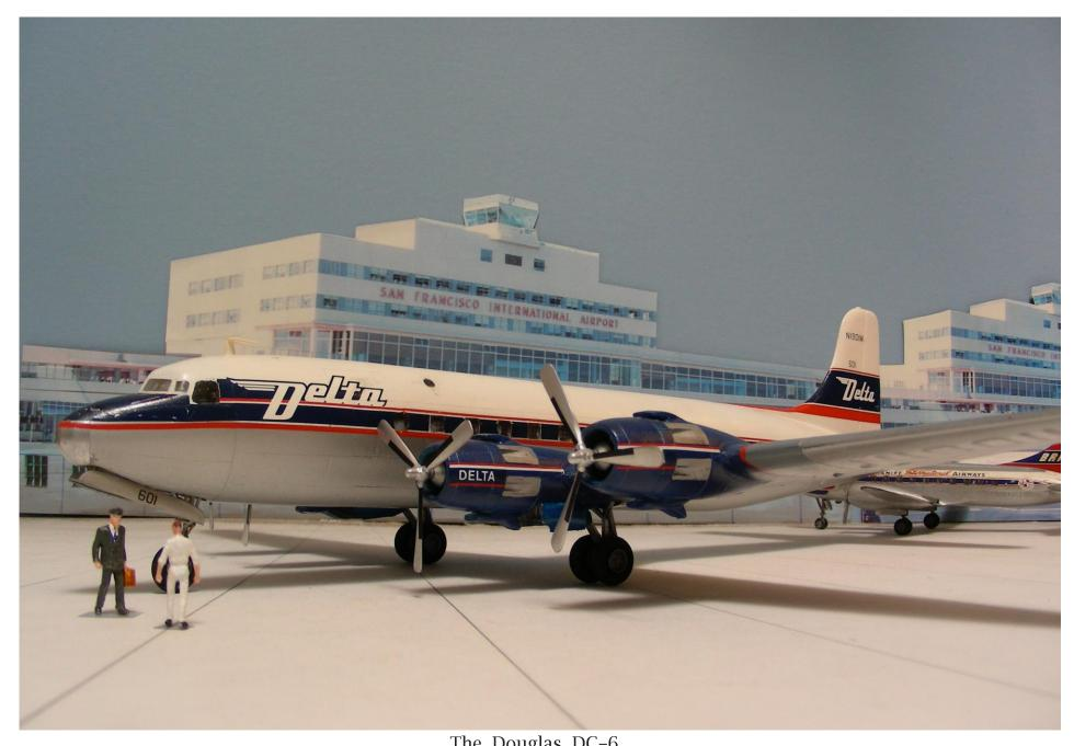
The Douglas DC-6 Converted Heller DC-6B, Pattern by Jim Lund. Next generation Douglas airliner, introduced in 1946, it had an enlarged, pressurized cabin and was a more powerful version of the DC-4/C-54 that preceded it.
