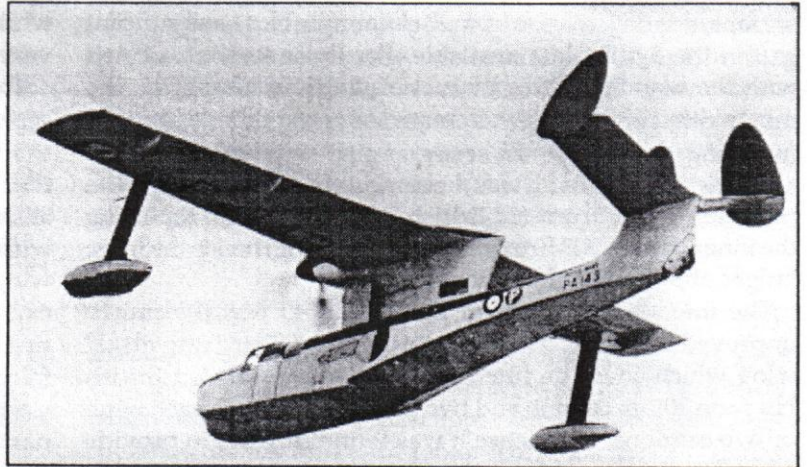
The Seagull's unique triple tail configuration came about late in the test program.
