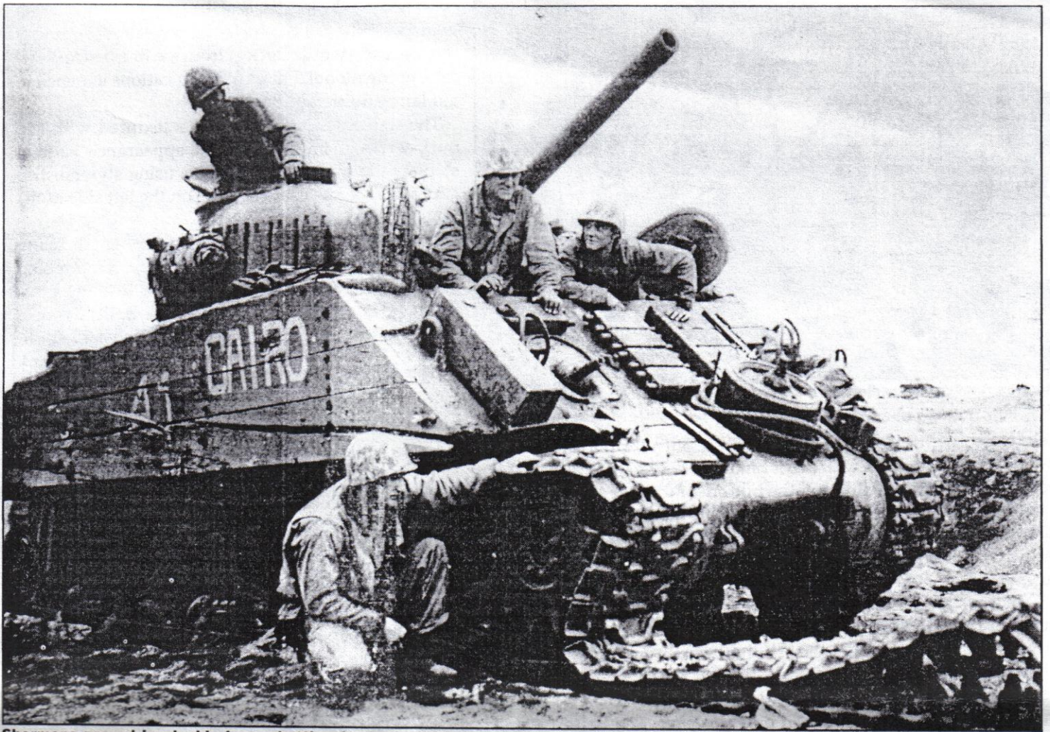
Shermans proved invaluable in combatting Japanese bunkers and fortified emplacements. This M4A2 displays the wood and concrete supplemental armor used late in the island-hopping campaign.
