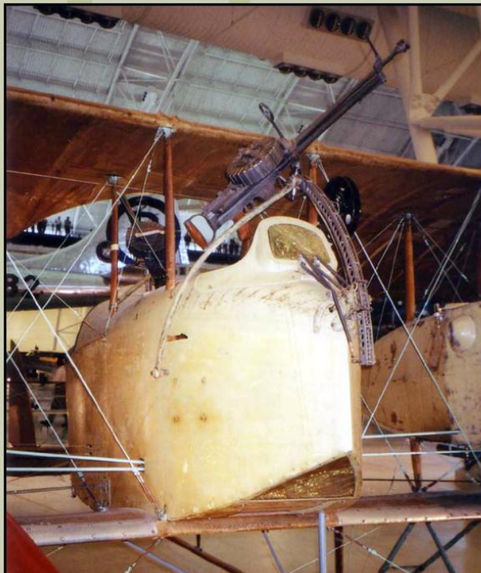
The center nacelle of the twin engine Caudron G.4 with its gun track. The pilot sat in the rear while the observer rode up front.
