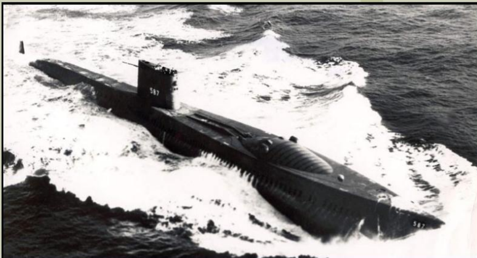
Halibut was nicknamed "The Bat Boat" and her super secret hanger "The Bat Cave." Her hull shape was too noisy above moderate speed making the design a dead end.
