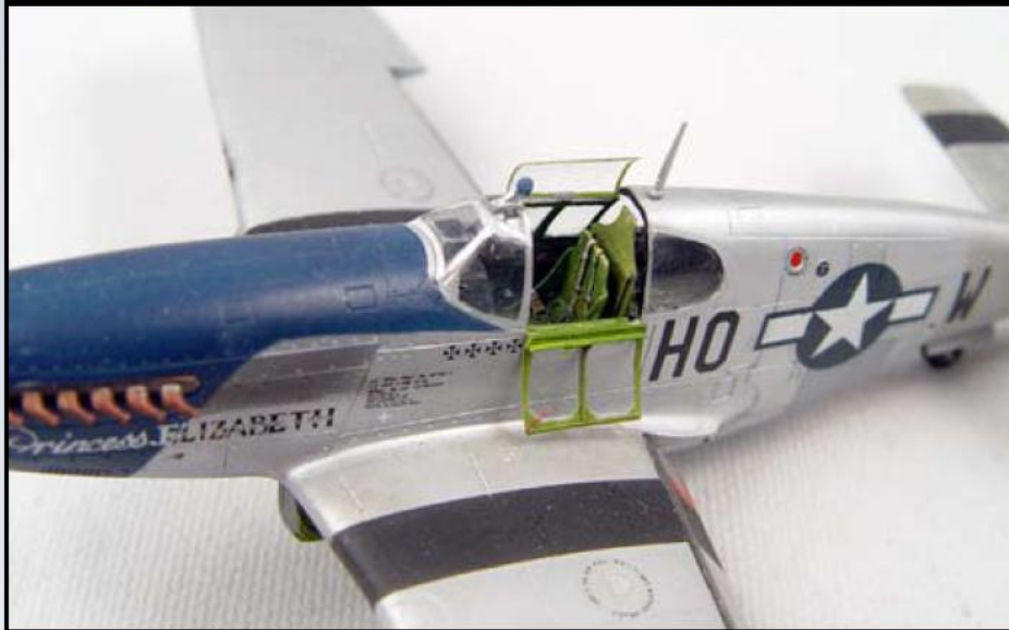
Although the Academy kit had a decent cockpit, Chris added more detail by using the Hawkeye Models P-51B interior. This was painted with Testors' Model Master aircraft interior black, then over-painted with interior green shot from above to create a shadow effect.
