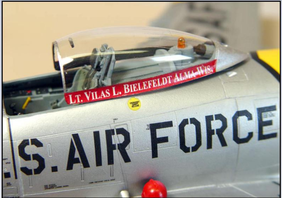
To replicate the canopy markings on FU-351 at the time of the gunnery meet, John created decals using Adobe Illustrator and a laser printer. Much of the turtle deck detail was made from strip styrene.
