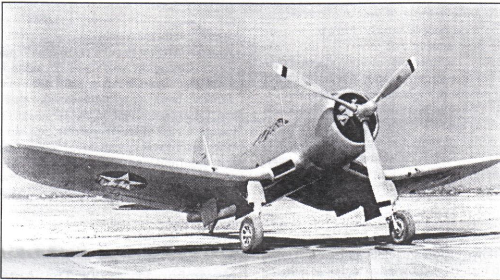
The first Corsair had different armament, a cockpit set farther forward, and small bomb bays in the wings for air-to-air mines. Still, there's no mistaking the prototype as anything but a Corsair .
