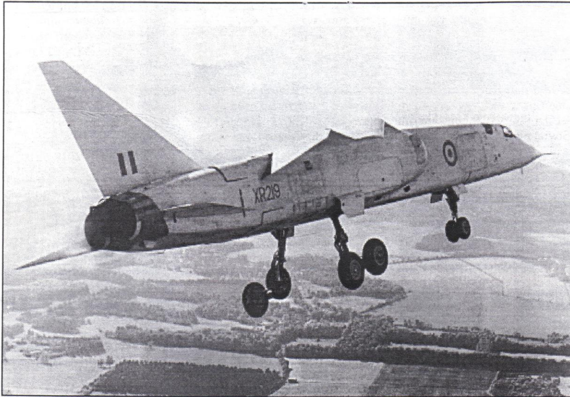
To meet the requirement for take-off and landing from unprepared strips, the TSR.2 had a unique undercarriage that hung in a gawky manner before touch-down. Problems with vibration in the gear on landing were never solved.
