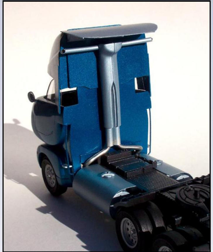
Plastic card was used to form the back wall of the cab. The rear wheel wells were also filled with plastic card.
