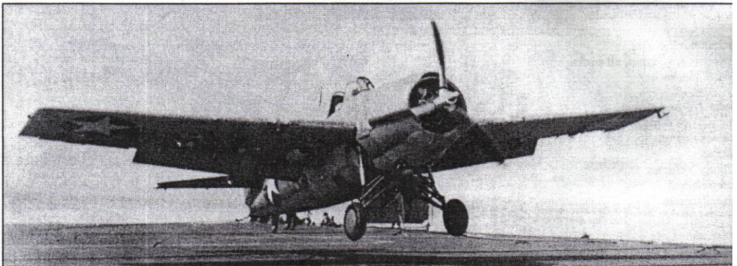
Besides the folding wings, the F4F-4 could be distinguished from the -3 by the small pitot probe on the left wing and the simplified windscreen.
