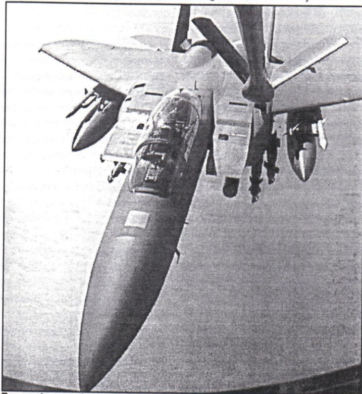
Boomer's-eye view of an F-15E during a peacekeeping mission over Bosnia, armed with four Laser Guided Bombs and four AMRAAMs.
