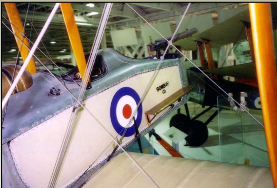
Note how light the ribstitch tape on the top of the wing is on this Vickers FB-5.
