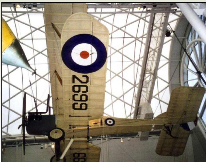
The Imperial War Museum’s BE-2—Notice what complex paint work it would take to accurately reproduce its appearance. You would need a soft-edged band to represent the shadows of the ribs with a sharp-edged light stripe for the tape.
