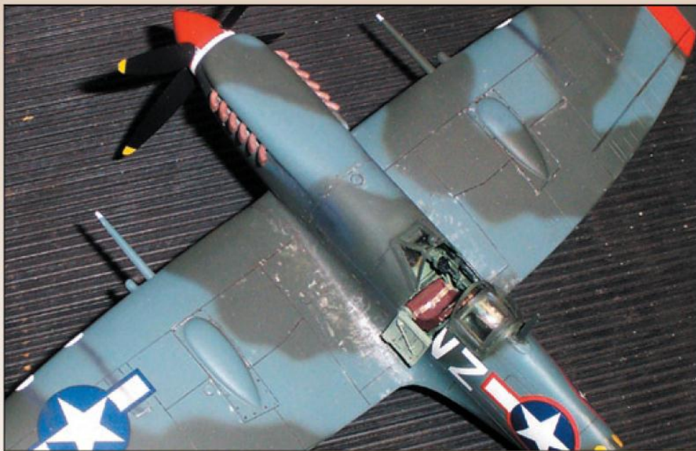
The cockpit was detailed with dressed up Tamiya parts and strip-stock. The door was scratch built with sheet styrene and stretched sprue for a more scale appearance.
