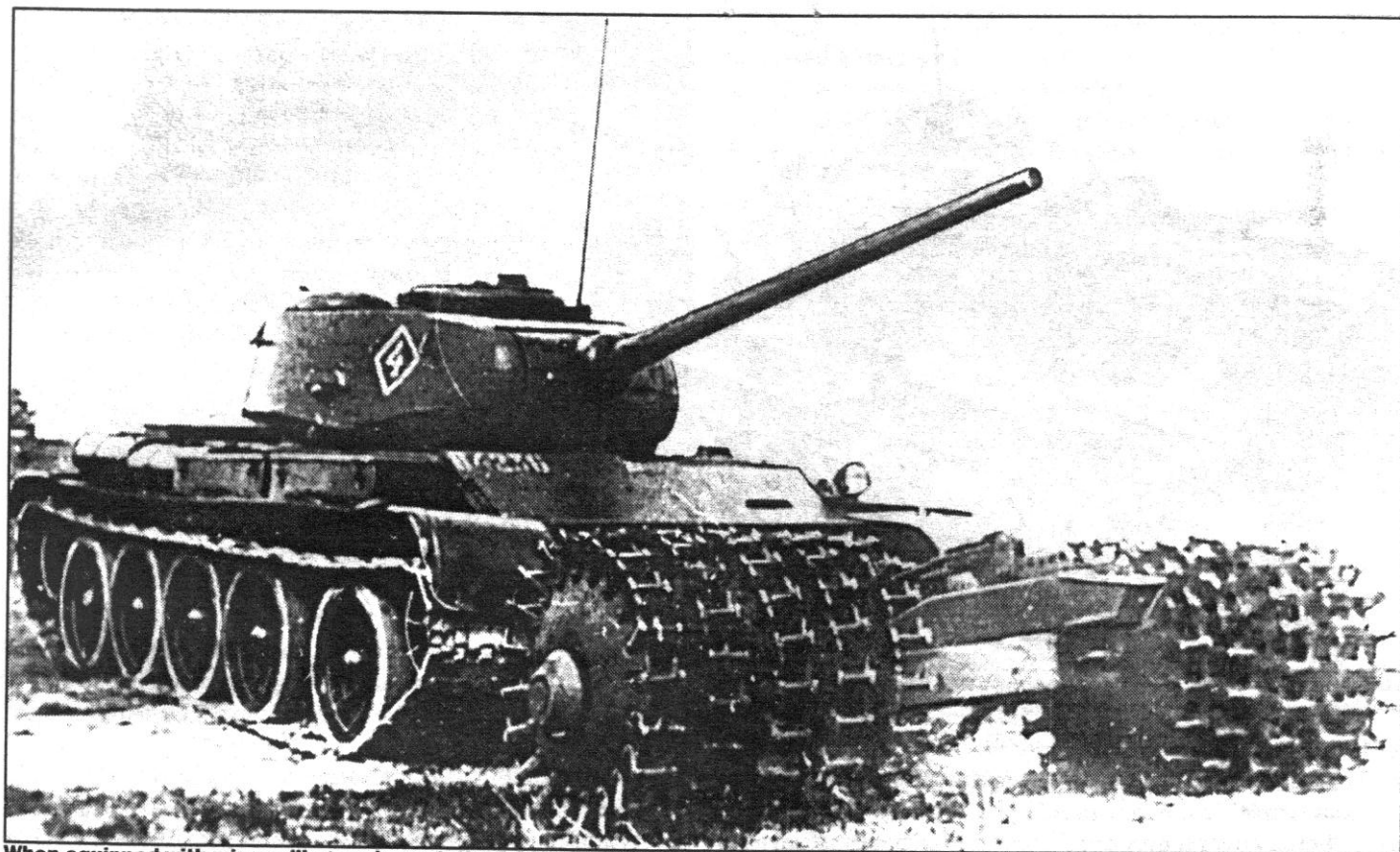
When equipped with mine-rolling equipment, the T-44 turned into the PT-44. Some of these tanks remain in use even today with second-line Russian combat units.
