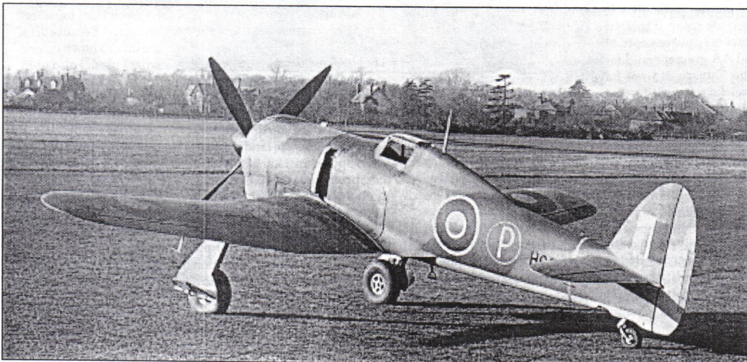
The Tornado achieved a top speed of 402 mph, but the thick wing employed didn't allow it room for improvement, just as in the case of its stablemate, the Typhoon .
