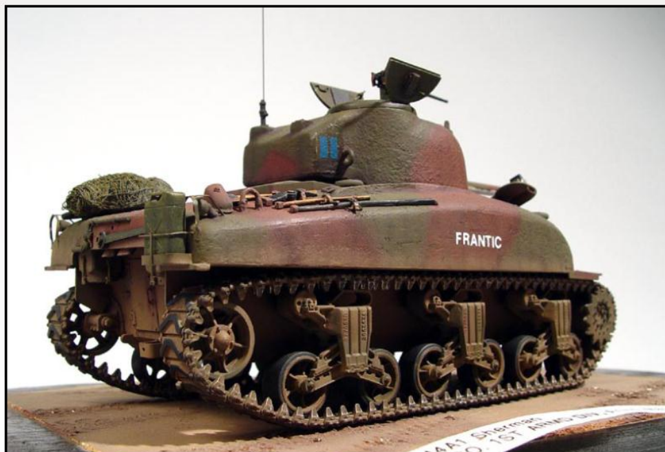
Laramie built his Sherman's running gear in such a way that he can install the wheels into the bogeys during the kit's final assembly. Laramie added bolt heads that he created with his punch and die set to the bogeys.
