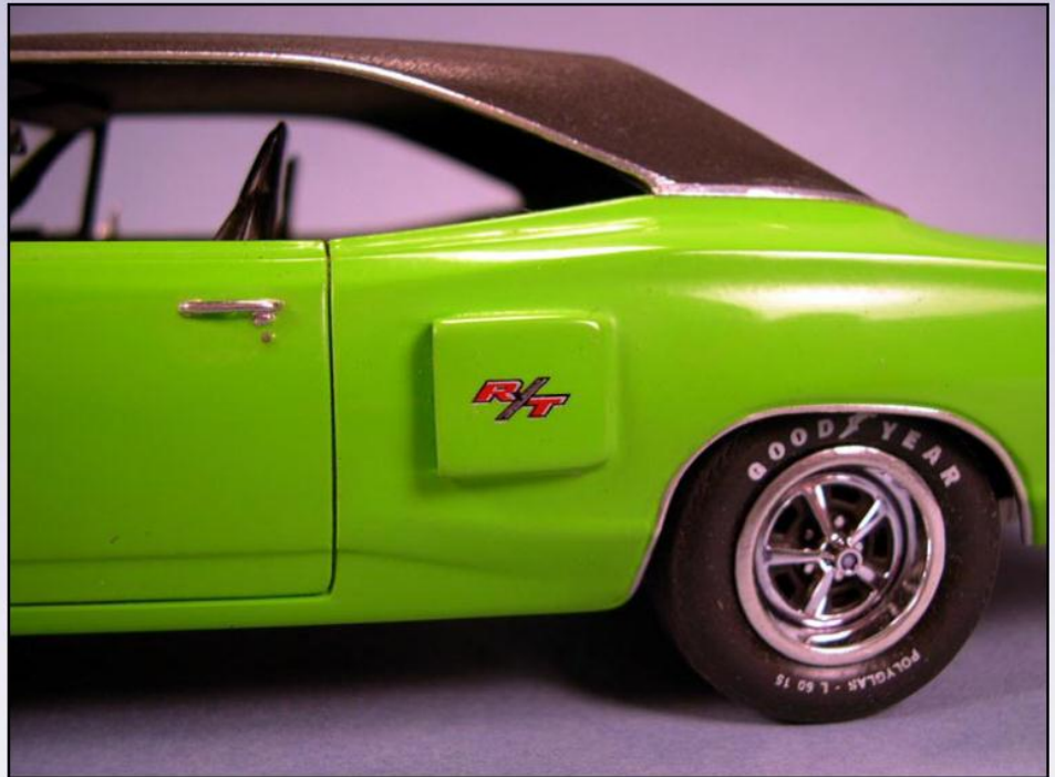
Andy built the side scoops from 0.060" and 0.030" sheet styrene. The R/T decals came from the Monogram '69 Charger kit.
