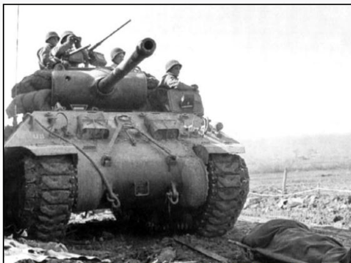
An M36 near Guidekirch, France March, 1945. Notice the Sherman style gun lock on the front of the hull.
