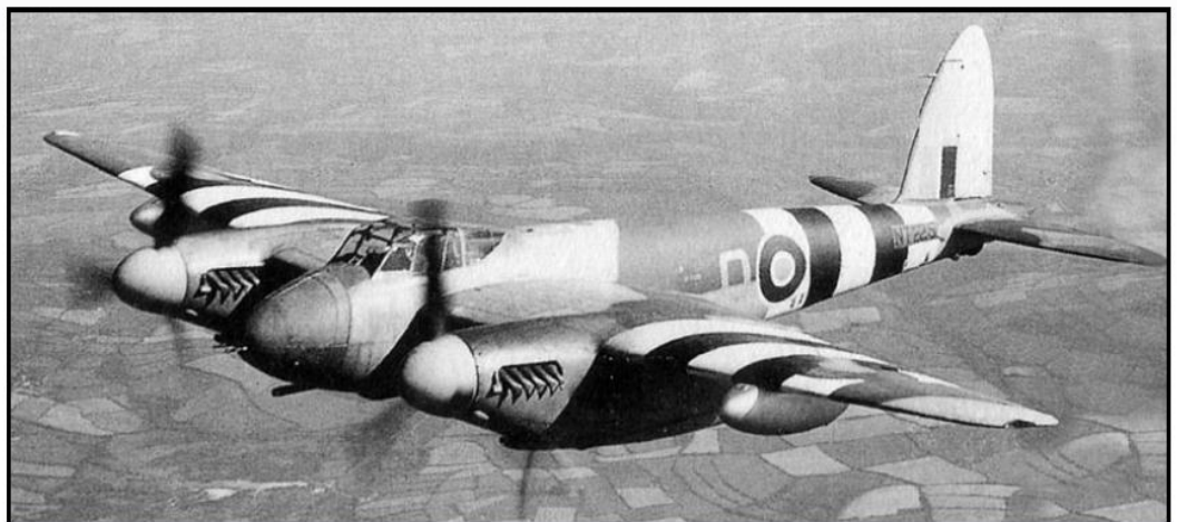
Another image of NT225. The Molins gun can be seen poking out from under the nose. The anti-shipping gun replaced the four 20mm cannon.
