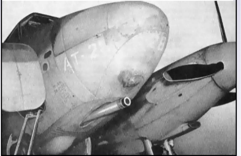
The aircraft version of the Molins gun with autoloader (top). The business end of the Mk. XVIII "Tsetse" with the Molins gun (bottom).
