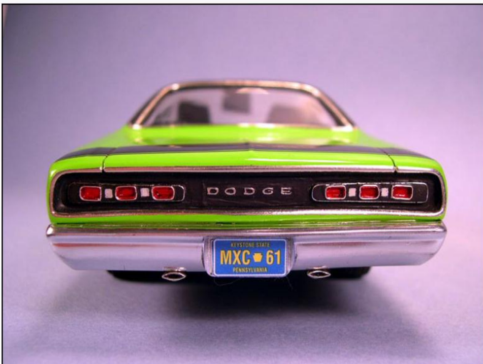
The tail light panel was built from Evergreen sheet. The DODGE logo is from the Super Bee tail panel. The individual tail lights were made from 28 gauge wire wrapped around a jig carved from styrene rod.
