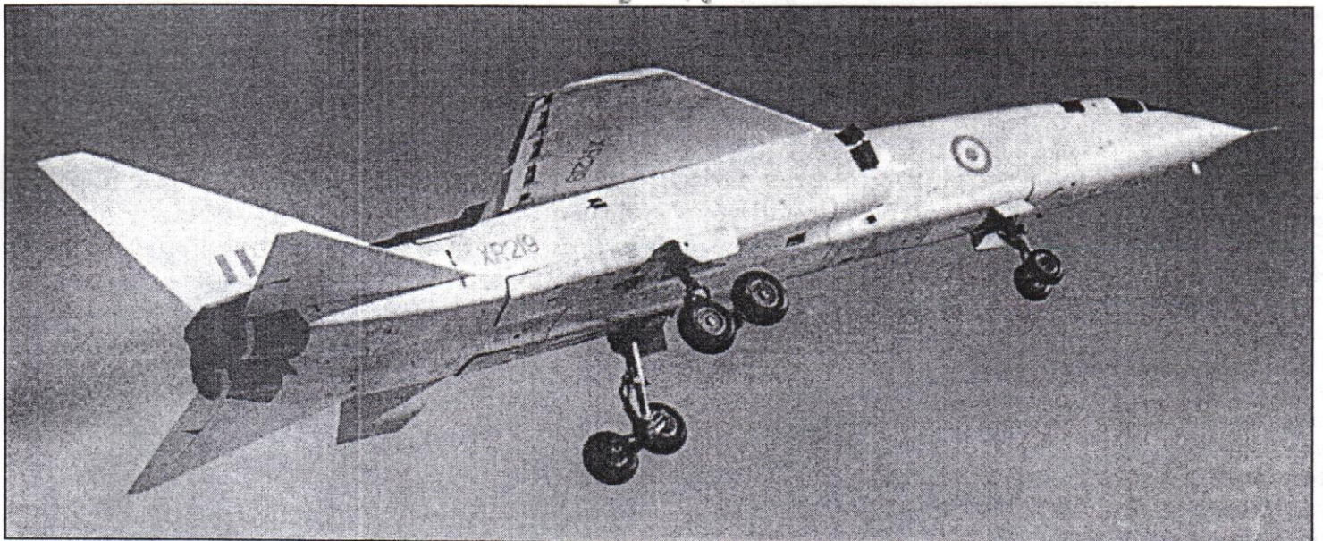
One of the areas to cause trouble in the test program was the landing gear, designed to operate from damaged or unprepared fields. On flight 5, pilot Roland Beamont almost lost control due to a vibration that was never quite resolved. Here, the unique offset struts are visible.
