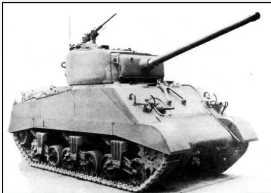
This M4A2 is equipped with the 76mm gun. It has the newer front hull that did away with the bulging hatches on the earlier hull. Additionally, the hatches were larger allowing the crew to get out more easily.
