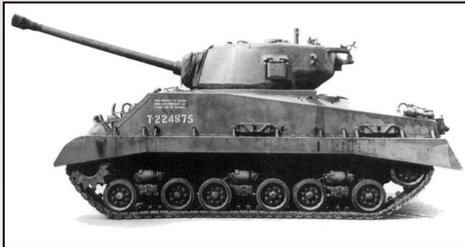
This M4A3 is equipped with the 76mm main gun. The hull is the welded/composite type and has the HVSS system.
