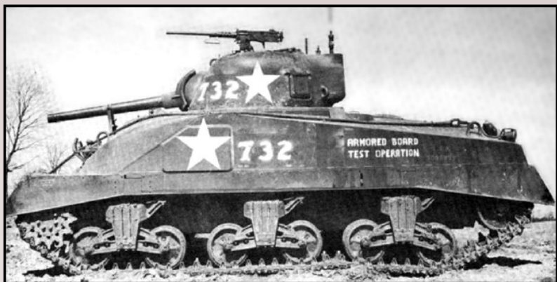
The M4A6 had a welded hull and the 75mm gun and the VVS suspension.
