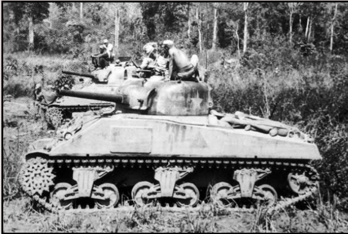
The M4A4 had a longer hull than other Shermans and the suspension is spaced further apart.
