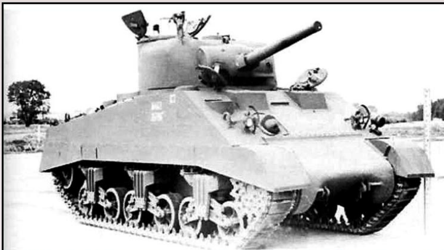
An M4A2 with the 75mm gun. This machine has the welded hull as well as welded-on armor in front of the driver and co-driver's hatches. The M4A2 was powered by the GMC 2 X 6 cylinder diesel engine.
