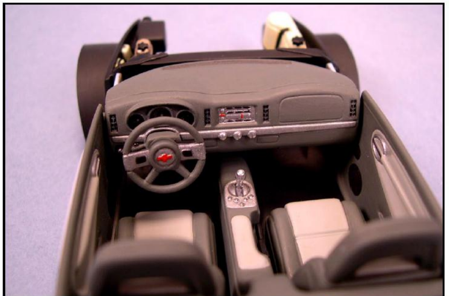
The interior is the kit plastic painted two tone gray - Humbrol #40 and #32. Details that were painted with aluminum and chrome silver with a black wash.
