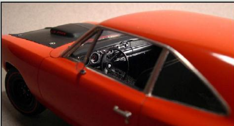
The column shifter is made from nickel plated electrical wire and the knob is epoxy. Andy also replaced the over sized turn signal. Yes, it was also made from electrical wire.
