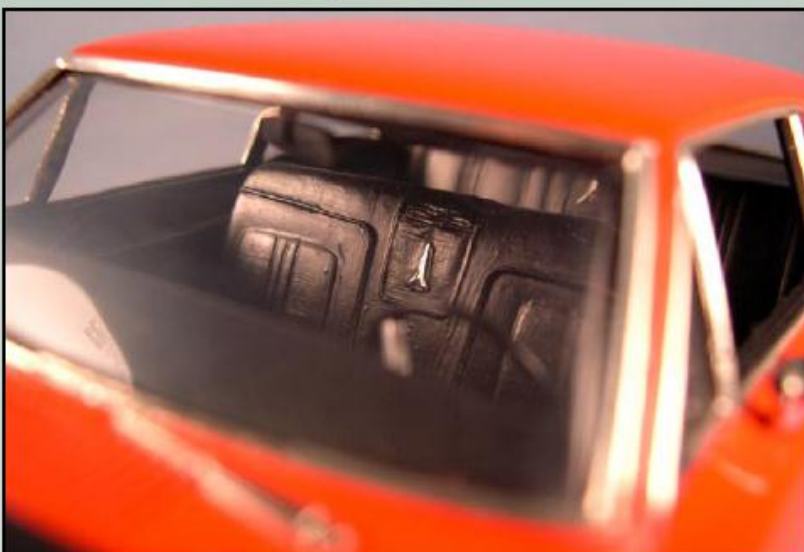
Andy converted the bucket seats into a bench seat using sheet styrene. The piping is electrical wire and the Dodge logo is the logo from the back seat embossed in aluminum foil.
