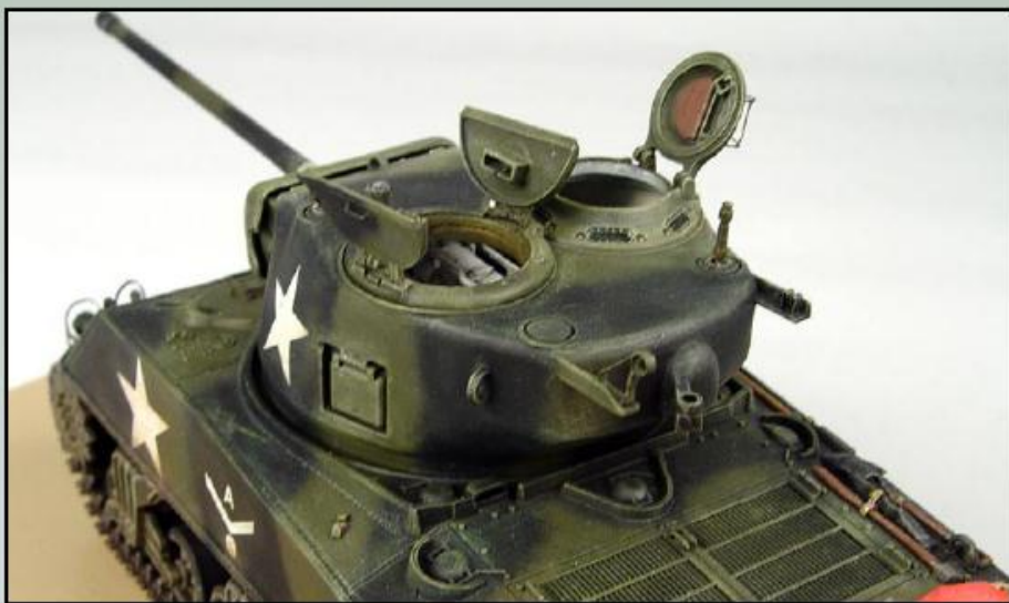
Laramie added casting texture to the sides and mantlet, and several photoetch details including periscope guards, roof mounted sight, stowage brackets and the .50 cal. stowage clamp, as well as several scratch built details.
