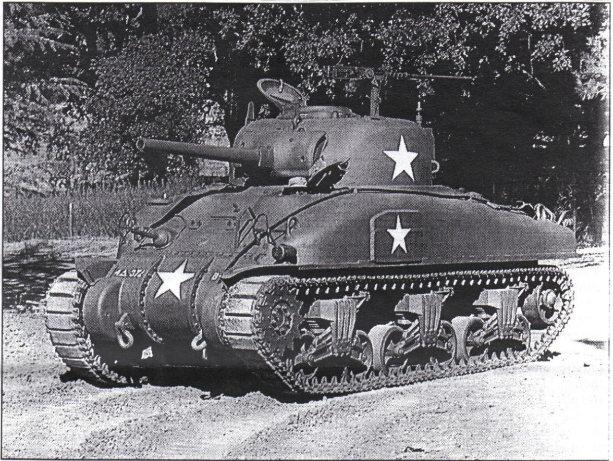
A cast-hulled M4A1 Sherman, retrofitted with applique armor. This version of the famous tank was powered by a Wright aero engine.
