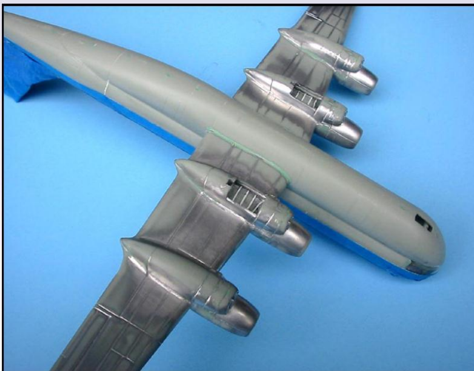
With all the putty sanded down, Bill's Stratocruiser is almost ready for paint. Bill used strip styrene to create some stringer detail in the gear wells.
