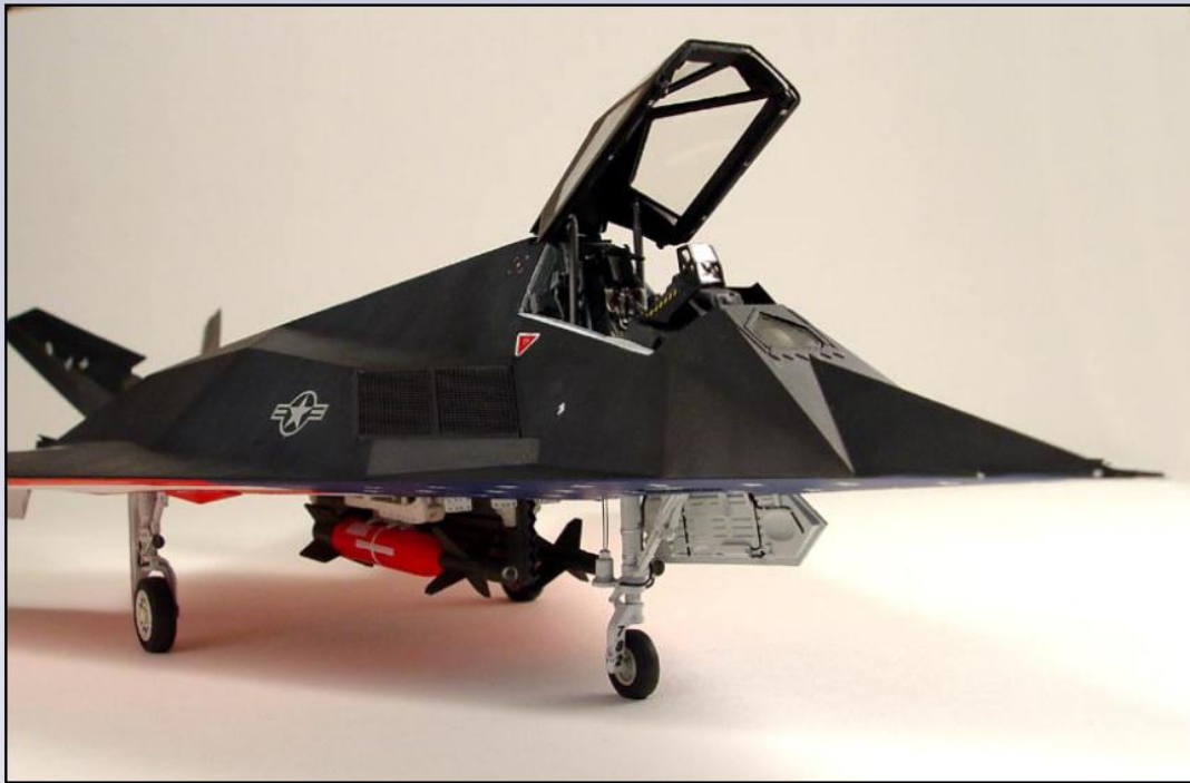
John used aluminum foil and car model spark plug wire to plum the landing gear. The 782 decal on the front landing gear was printed on John's ink jet printer.
