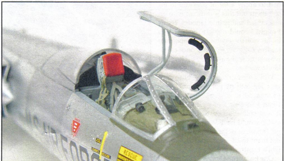
The rearview mirrors are from a Reheat photo-etched set. The area forward of the instrument cluster and the gun sight are part of the Aries cockpit set and added much detail to an area that is a bit marginal with the kit parts.
