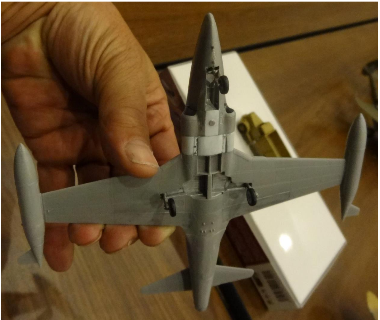
Lou Orselli's T-33 dodged the problem with part 33A by losing it and he had to make his own. Lou battled the step between the tail and forward fuselage and has his model ready for paint.
