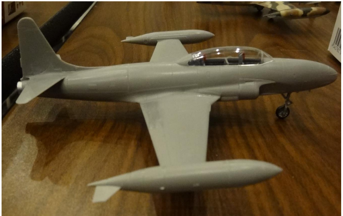
Lou Orselli's T-33 dodged the problem with part 33A by losing it and he had to make his own. Lou battled the step between the tail and forward fuselage and has his model ready for paint.
