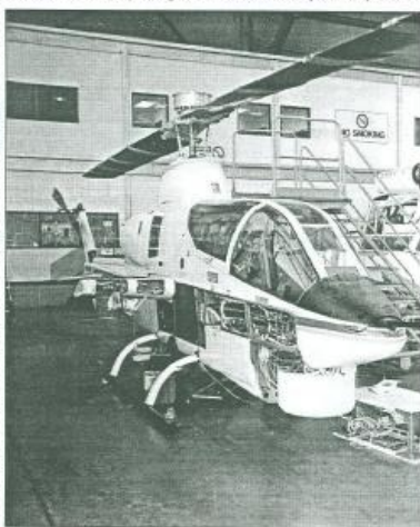
NASA/Ames' first Huey Cobra, an AH-1C, wired with sensors on the rotor to detect sound. This Cobra was at Ames until 1980.
