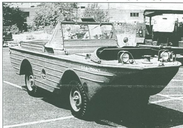
The Ford GPA, known as the 'Seep' by its crews, was essentially a boat hull mated with a Jeep chassis.
