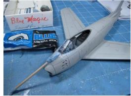
The model is assembled, then I give it a wet wash with diluted XF-1 mixed with Denatured Alcohol, (DA). This old method of mine sure shows up the sanding flaws and any missing panel lines that need to be
