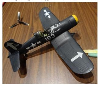
model down and seeing when the horizontal stabilizers "touch" the wing. If the two stabilizers touch at the same time, you're lined up properly.
