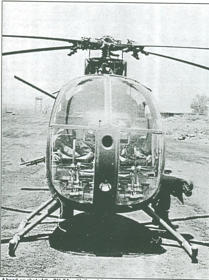
A head-on shot of the OH-6A, with the minigun visible on the right and the crew chief's M-60 on the left. The size of the windscreen shows why it's a problem for modelers.
