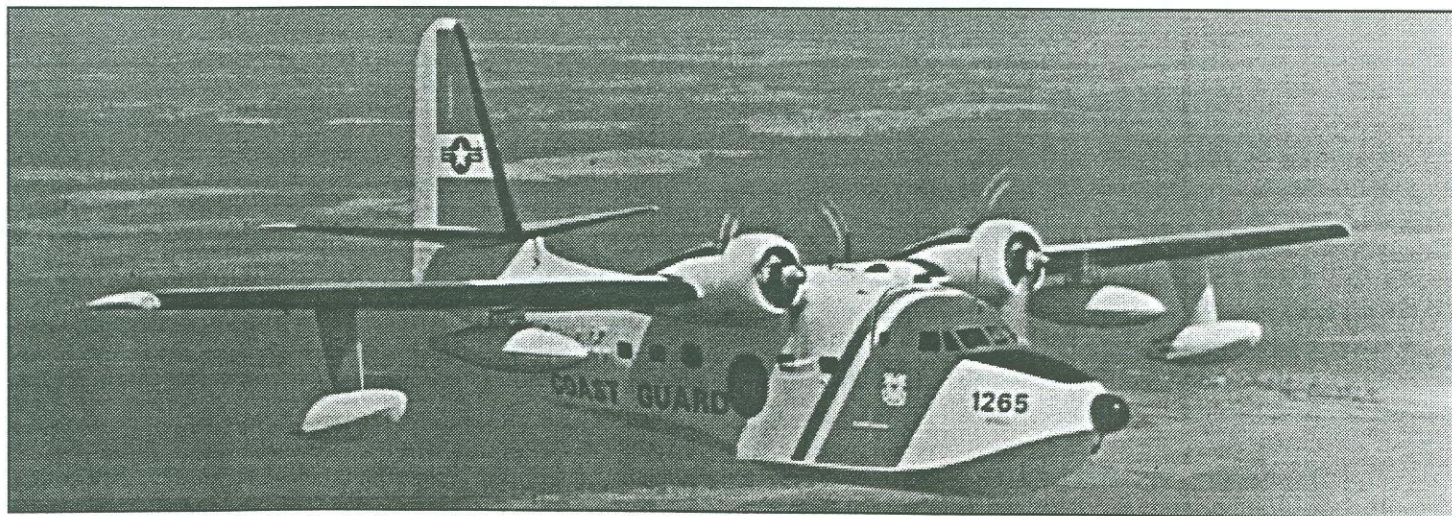
Lovely airborne shot of a Coast Guard Albatross , motoring through the air thanks to its twin R-1830 engines.
