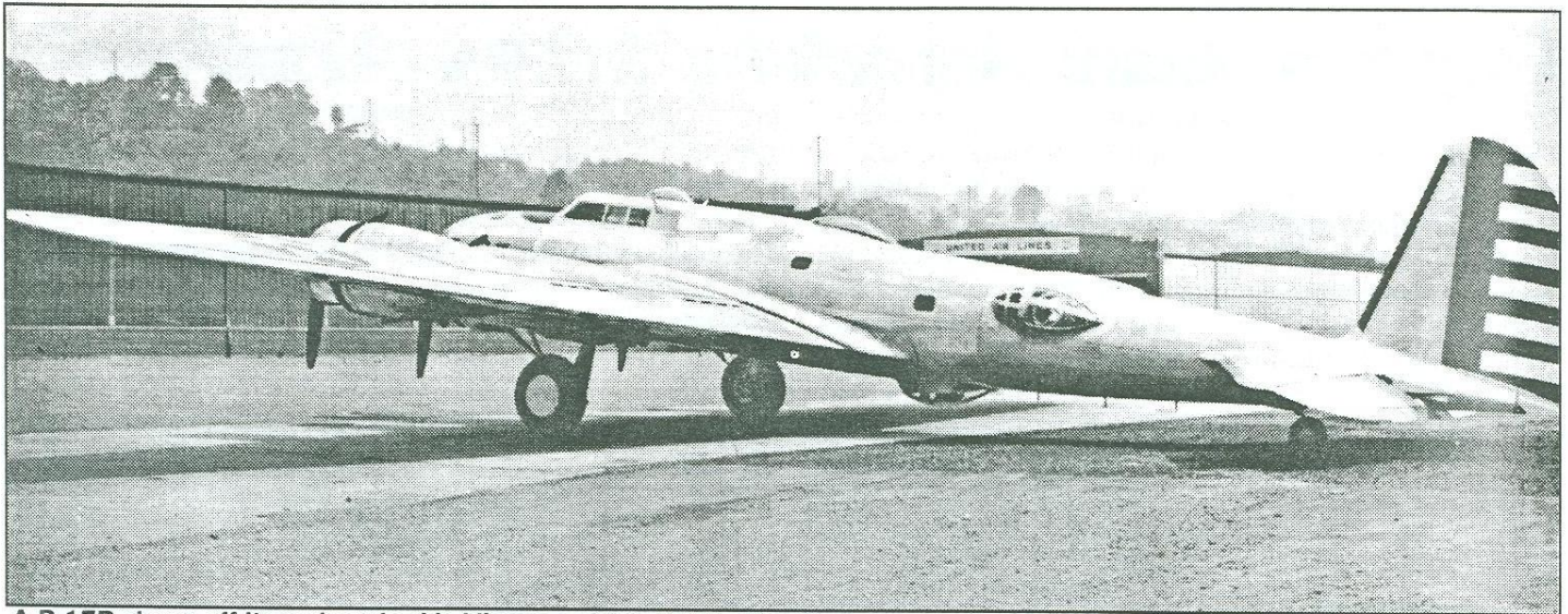
A B-17B shows off its early-style side blisters and "shark" fin. The Koster conversion provides replacements for many of the late B-17 components, including the tail and rear fuselage.
