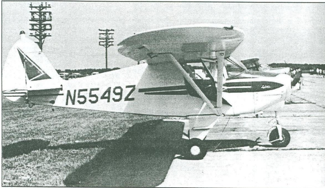
This Tri-Pacer shows off the spindly look that resulted from the stretching of the old Cub design.
