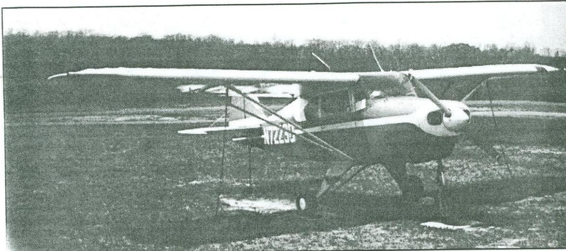
A Piper Tri-Pacer , the successor to the Pacer , at rest. The plane's tricycle gear was a departure from its taildragger forbearer, the Piper Cub .
