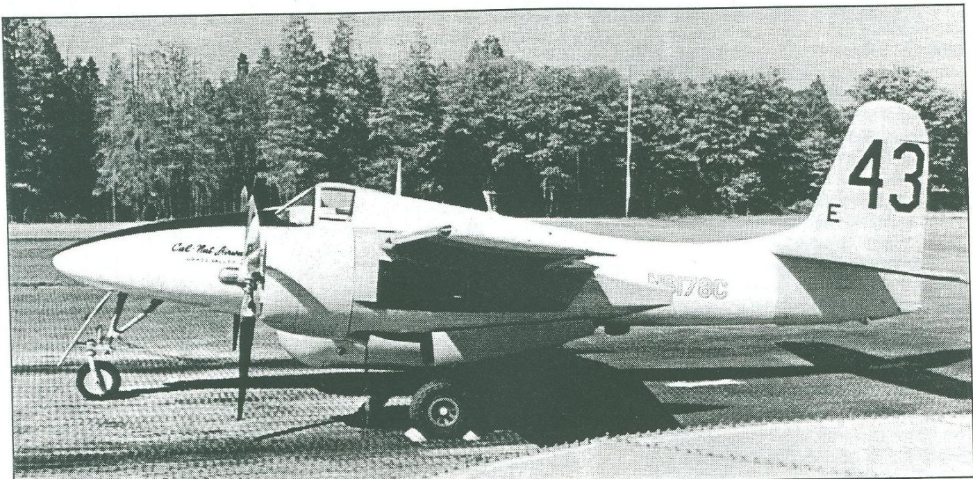
An overall white Sis-Q firebomber in profile. Note the black anti-glare panel. This Tigercat is a later F7F-3 model with the tall tail.
