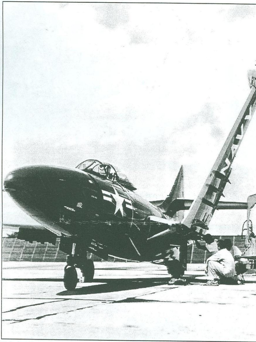
This head-on view shows the tell-take bulged intake, wing fence and tall tail characteristic of Dash-5 Panthers.
