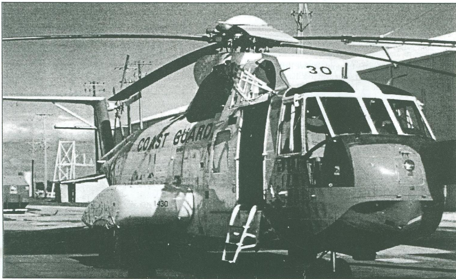
A Coast Guard Pelican on the ramp at USCG Air Station Clearwater, Florida. Note the gap between the fuselage and sponson.
